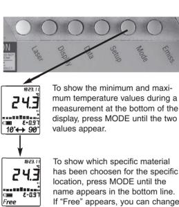
To show which specific material has been choosen for the specific location, press MODE until the name appears in the bottom line. If "Free" appears, you can change the emissivity settings by using the Emiss, button, when not in LOG mode. See chapter The Emiss, button!
