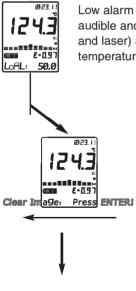
Low alarm (LoAI) generates an audible and visual (flashing LED and laser) alarm if the temperature is below the setpoint.
