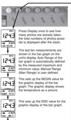
CYCLE allows the adjustment of the display interval of the bar
