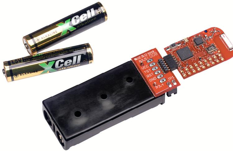
Figure 2. eZ430-RF2500 Battery Board
