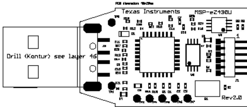
Figure 11. eZ430-RF, USB Debugger, PCB Components Layout
