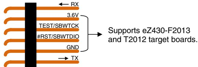
Figure 4. eZ430-RF2500 USB Debugging Interface 6-Pin Male Header
